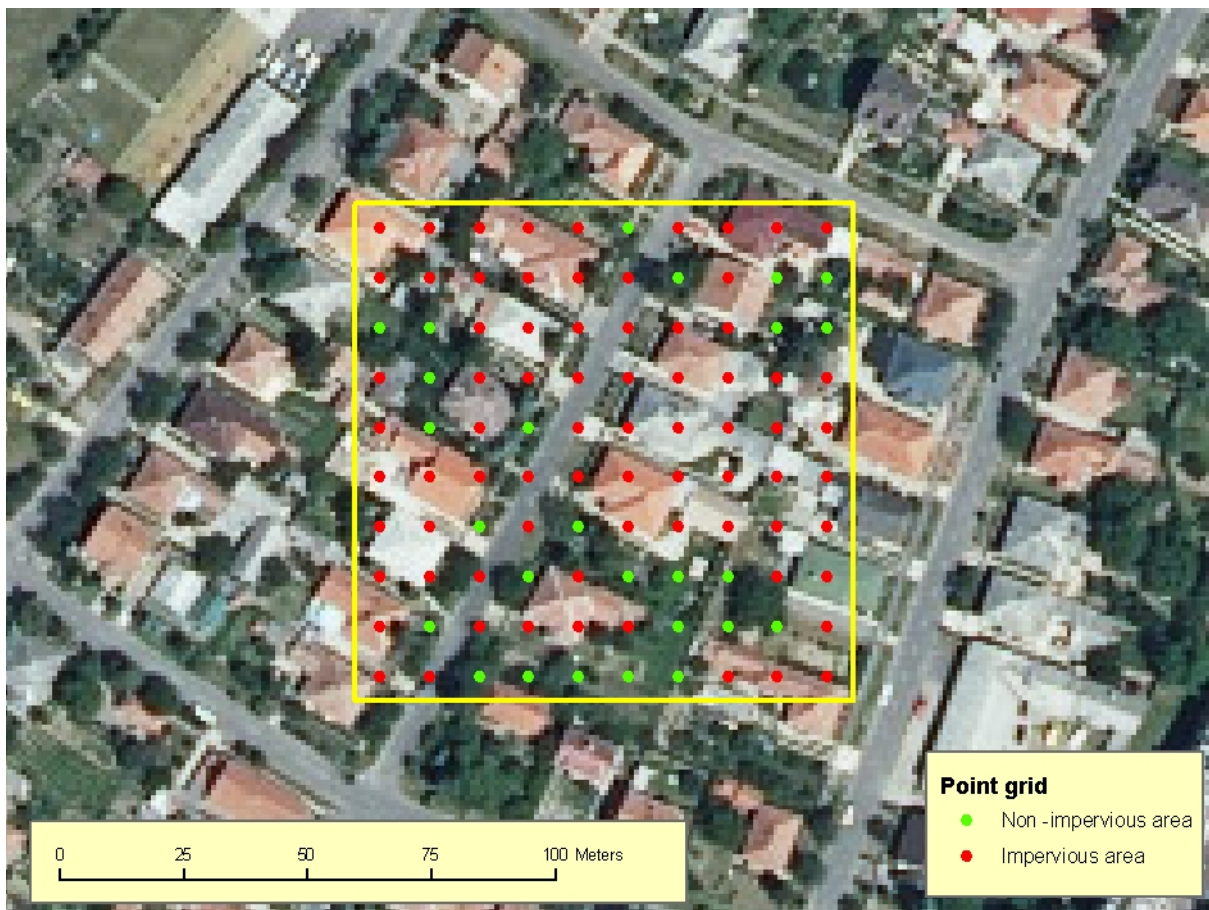
Figure 3: Visual interpretation of a sample observation (100 m x 100 m). By counting the impervious points out of the 100 points, the interpreter estimates sealing degree of the sample
