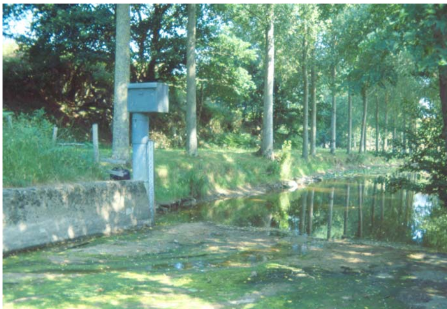
Figure 1: Example of dried out river at the gauging station, in relation with the presence of concrete section.
