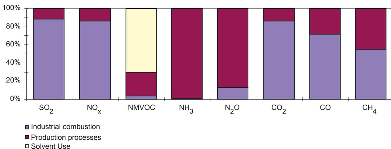
Figure 14 Distribution of the industrial emissions of GHGs and acidifying pollutants (Aeq) over combustion, process and solvent use emissions in 1990 (%).
