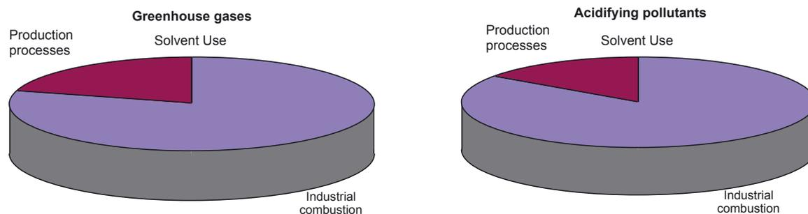
Figure 14 shows the contribution of combustion and process emissions to the industrial emissions of GHGs and acidifying pollutant. The major part of the environmental burden in these two themes is due to combustion (75 to 80%)
