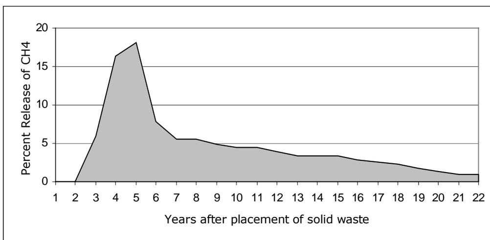
**Figure 5.1. Typical CH<sub>4</sub> Production Pattern in Solid Waste Disposal Sites**
