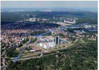
Cold air down-flow along the ventilation axis left free of buildings at Stuttgart-Vaihingen (City of Stuttgart).
