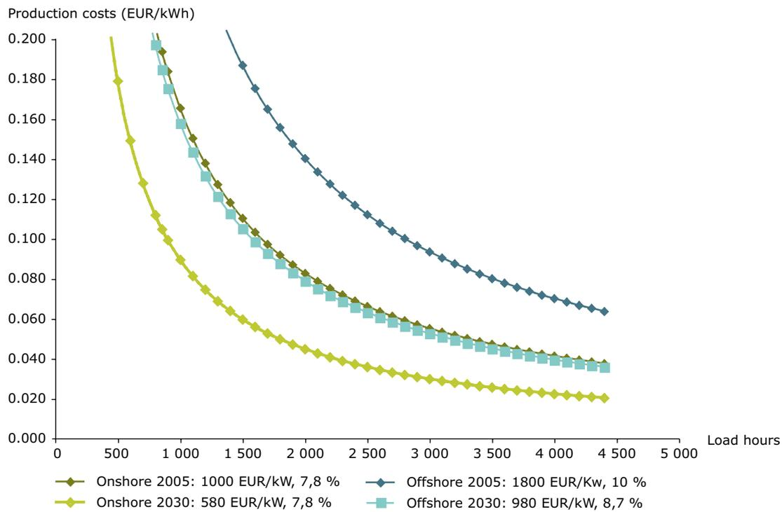
**Figure 6.4 Projected supply curves for European onshore wind energy in 2020 and 2030**
