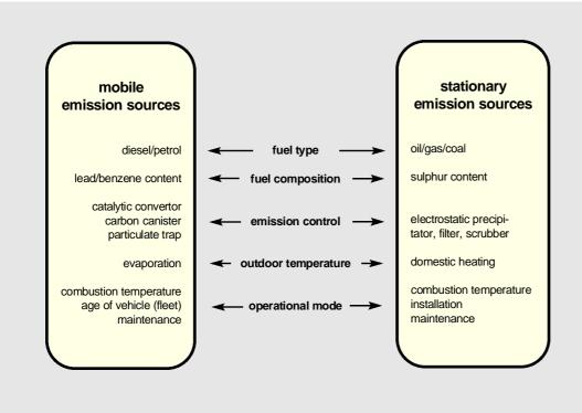
Figure 2.1 Key factors which influence emissions from combustion processes
