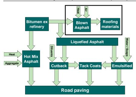
Asphalt roads are a compacted mixture of aggregate and an asphalt binder. Natural gravel, manufactured stone (from quarries) or by-products from metal ore refining are used as aggregates. Asphalt cement or liquefied asphalt may be used as the asphalt binder. The different techniques used in road paving with asphalt are discussed below in section 2.2 of the present chapter. Figure 2-2 shows the main processes, input and output in this process.
