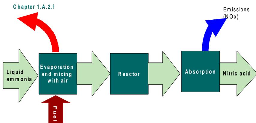
For nitrogen oxide (NO<sub>x</sub>) emissions, the relevant process units are the absorption tower and the tail gas cleaning units, e.g. selective catalytic or non-catalytic reduction (SCR, SNCR). Small amounts of NO<sub>x</sub> are also lost for acid concentrating plants.
