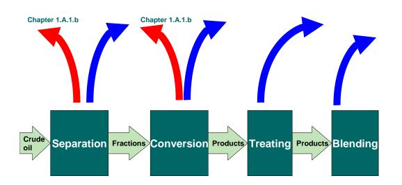
Diffuse emission sources are defined as NMVOC sources not associated with a specific process but scattered throughout the refinery. Fugitive process emissions are a subset of diffuse emissions and sources include valves of all types, flanges, pump and compressor seals, pressure relief valves, sampling connections and process drains. These sources may be used, for example, in the pipelines transporting crude oil, intermediates, wastes or products.
