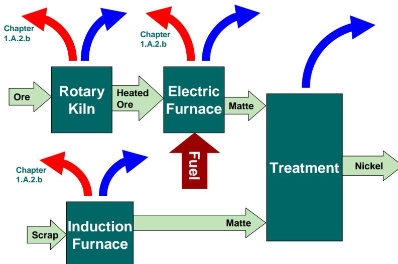
The energy consumed for the production of matte from sulphidic ores is reported to be in the range of 25–65 GJ per tonne of nickel for ores containing 4–15 % Ni. The energy consumed in the various refining stages is reported to be 17–20 GJ per tonne of nickel.
