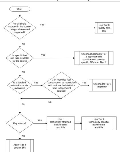
Figure 4-1 Decision tree for combustion in petroleum refining
