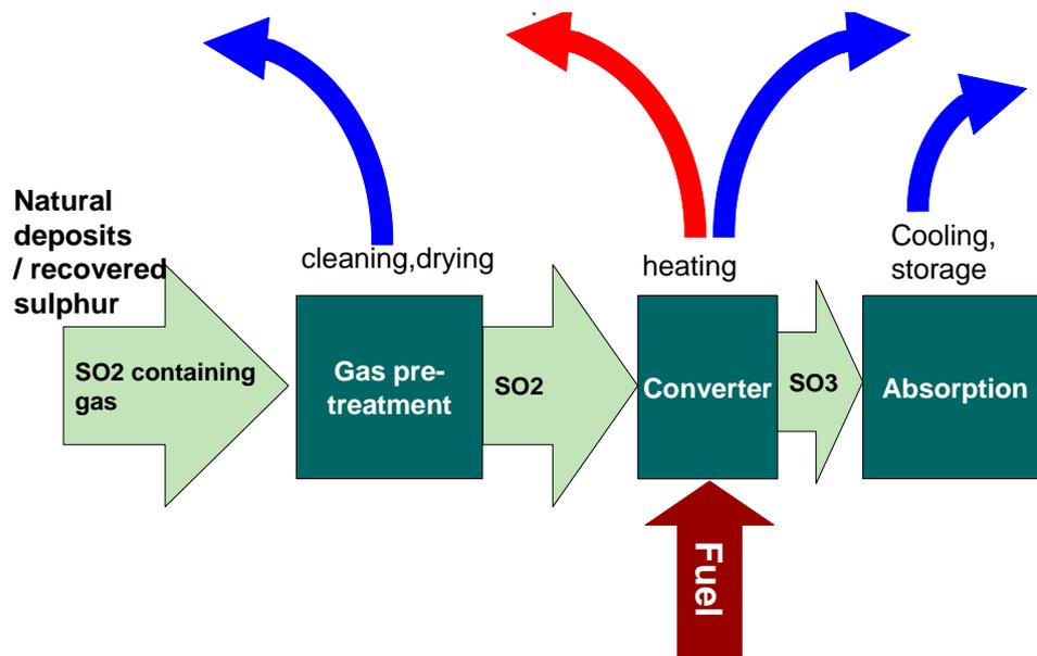
For sulphur dioxide (SO<sub>2</sub>) emissions the relevant process units are the cleaning of raw gas containing SO<sub>2</sub> (gas pre-treatment), the catalytic oxidation to sulphur trioxide (SO<sub>3</sub>) (converter) and final absorbing tower and scrubbers. Scrubbers may be installed for the cleaning of raw gas and behind the tail gas cleaning.
