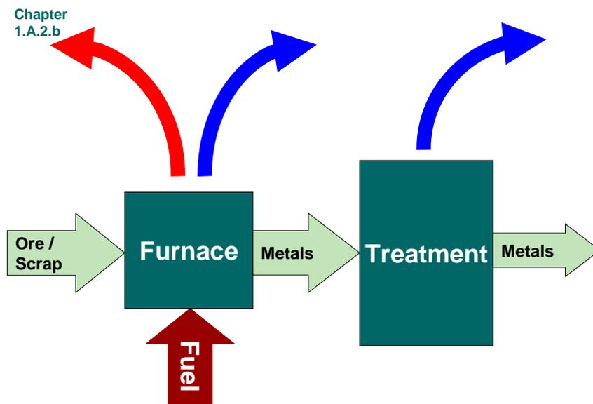
Figure 2.1 Generic process scheme for source category 2.C.7.c Other metal production
