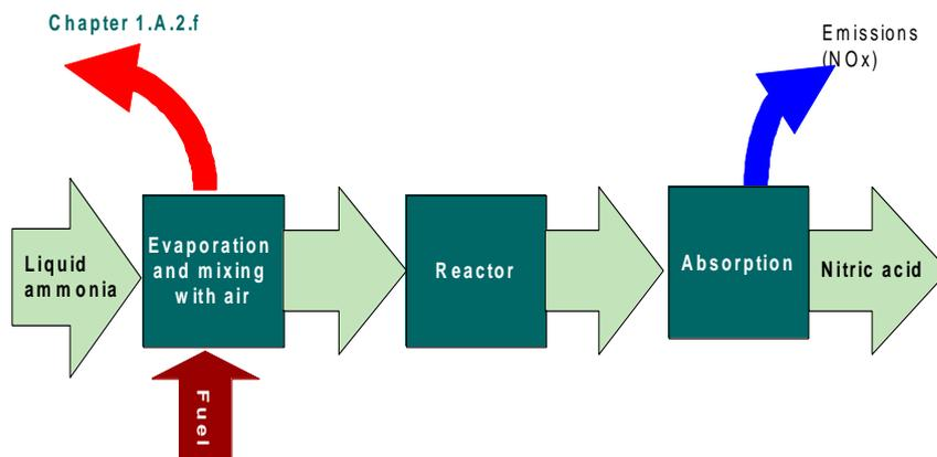
**Figure 2.4 Simplified process scheme of nitric acid production.**
