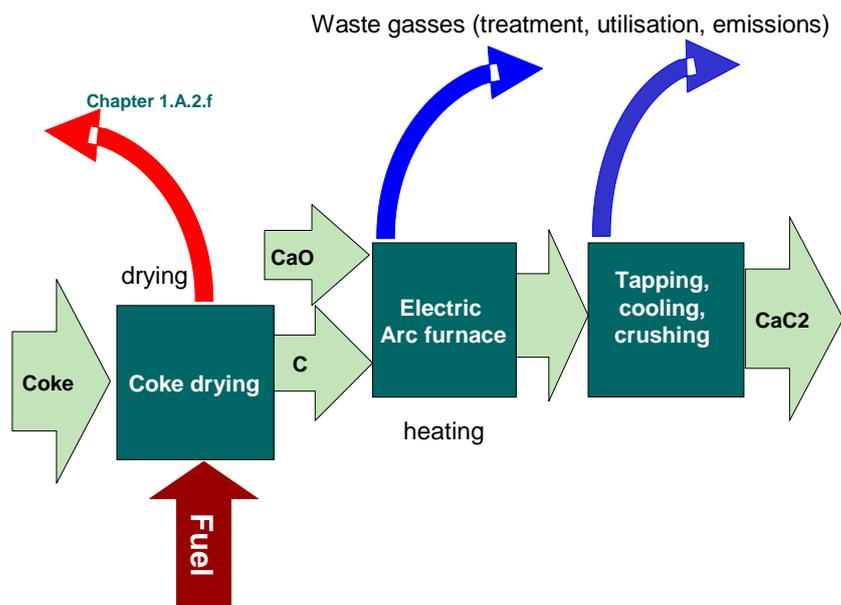
Figure 2.5 Simplified process scheme of calcium carbide production (EC, 2006c; US EPA, 1993).
