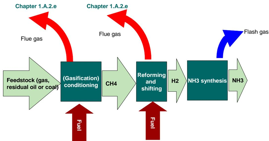
Figure 2.3 Simplified process scheme of ammonia production.
