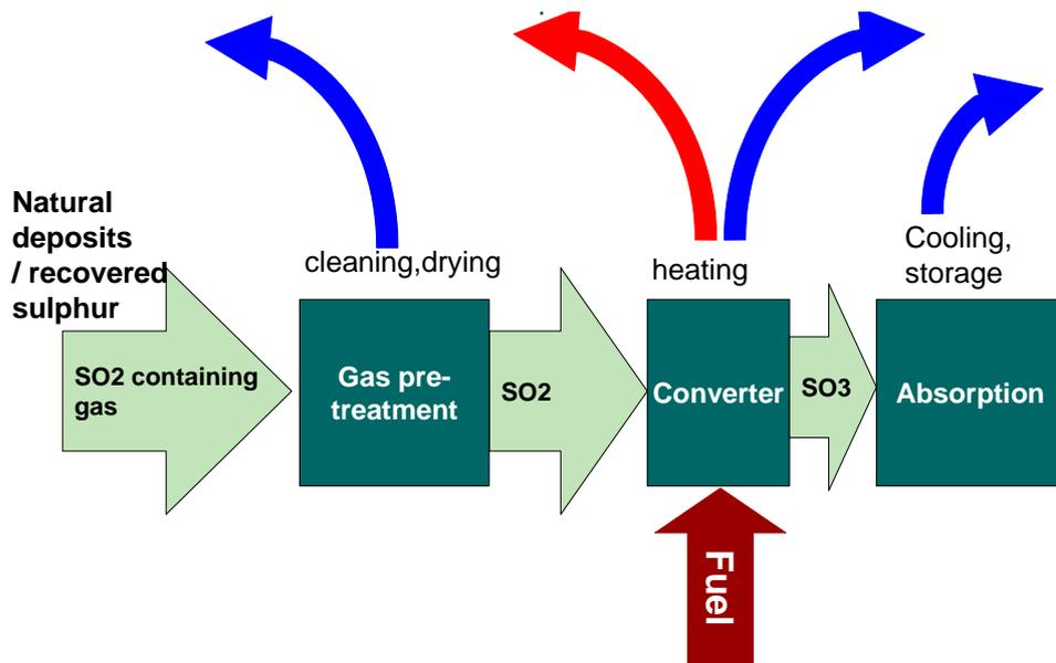
**Figure 2.6 Process scheme sulphuric acid plant.**
