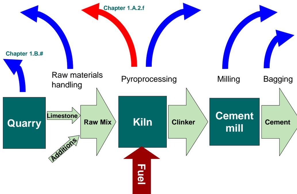
**Figure 2.1** Production of cement. Combustion emissions are indicated in red, process emissions are indicated in blue. Emissions from quarrying are addressed in chapter 1.B.1.a and those of combustion in chapter 1.A.2.f.
