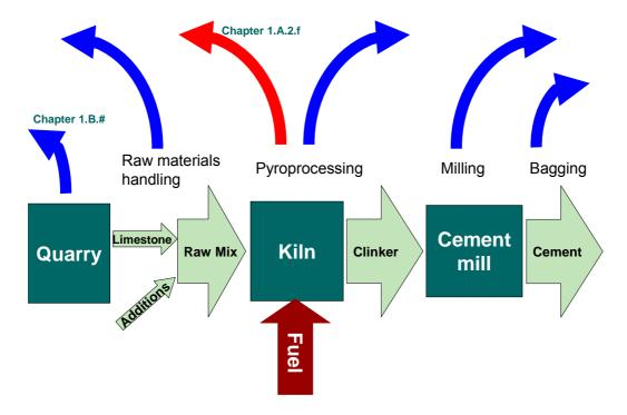
Figure 2.1 Production of cement. Combustion emissions are indicated in red, process emissions are indicated in blue. Emissions from quarrying are addressed in chapter 1.B.1.a and those of combustion in chapter 1.A.2.f
