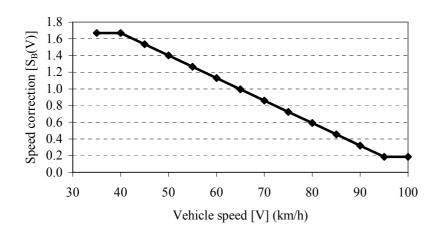
Figure 3–3 Speed correction factor for brake wear particle emissions
