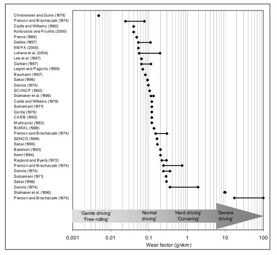
Figure 2-1 Wear factors for light-duty vehicle tyres (Boulter, 2005). 'vkm' = 'vehicle-km'
