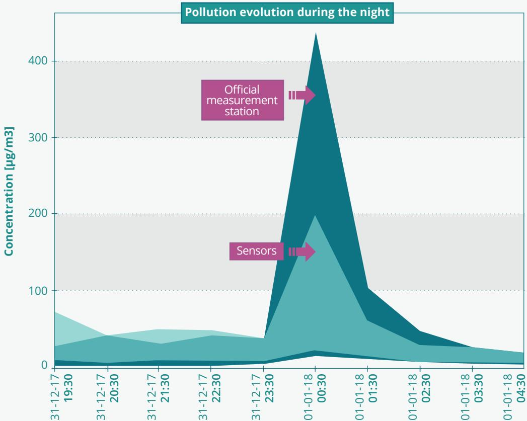
**Note:** The official data are available only on an hourly average basis, while the sensors report every minute. Comparing the concentration ranges between the 10<sup>th</sup> and 90<sup>th</sup> percentiles, i.e. the range where 80 % of the data are located, showed that the hourly average values of the official measurements were higher.
