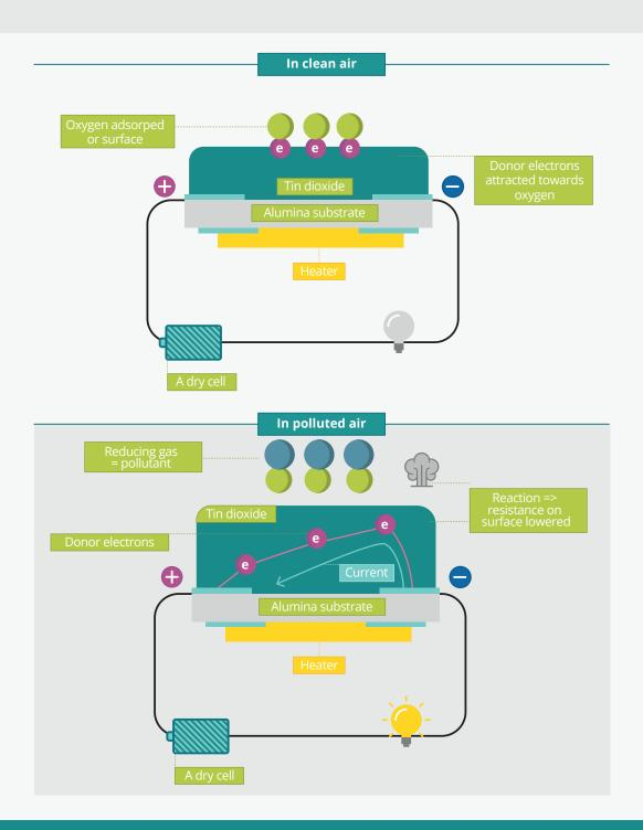
Based on: © FIGARO Engineering Inc., Japan. Note: Low-cost; around 10 to 15 Euro for a sensor (EC, 2019b).
