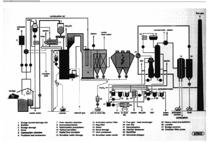
Process scheme of the sludge incineration plant of Dordrecht (the Netherlands) *Courtesy: Lurgi*  fluidised bed systems, which tend to be easier to operate (see Figure 8.1).
