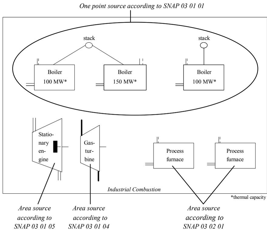
**Annex 2:** Determination of SO<sub>2</sub> emission factors (flow sheet, for description see Annex 3)
