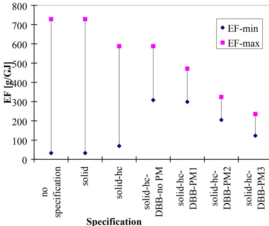
**Figure 3:** Ranges of NO<sub>x</sub> emission factors for the combustion of pulverised coal
