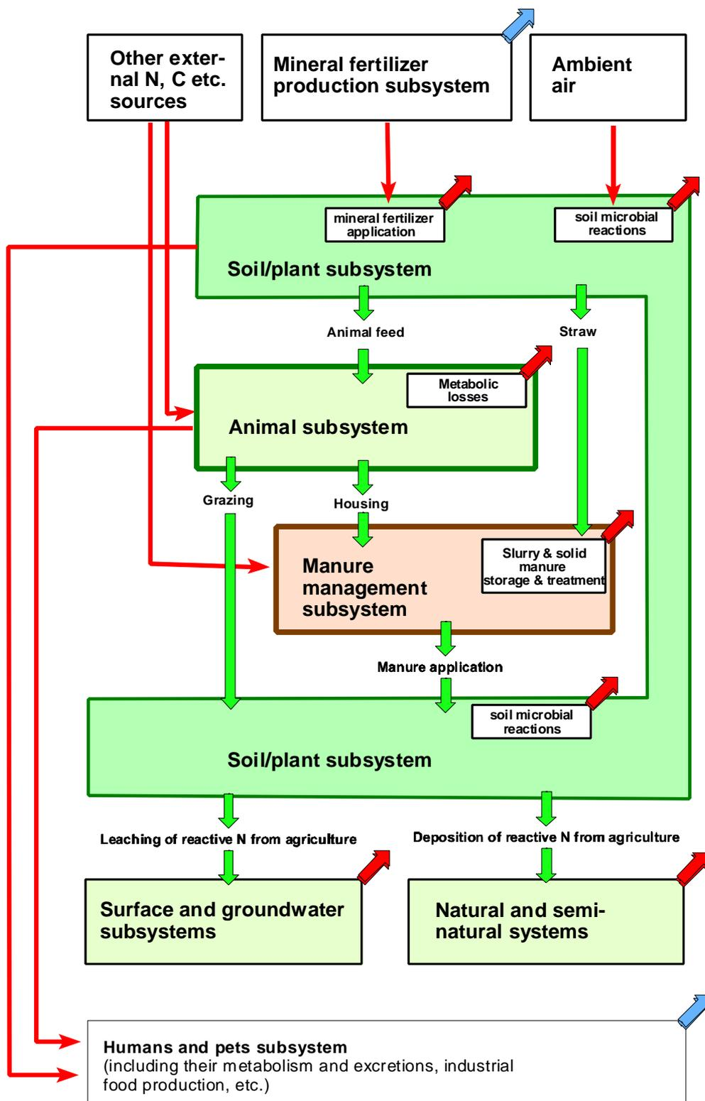
**Fig. 1:** Mass flows considered in the EMEP/CORINAIR Guidebook Chapter 10 (Agriculture): Red arrows: mass flow between external sources and sinks and the agricultural subsystems; broad red arrows: emissions to the atmosphere. Green arrows: fluxes between agricultural subsystems. Blue arrows: emissions not accounted for as agricultural emissions (Dämmgen et al., 2003)
