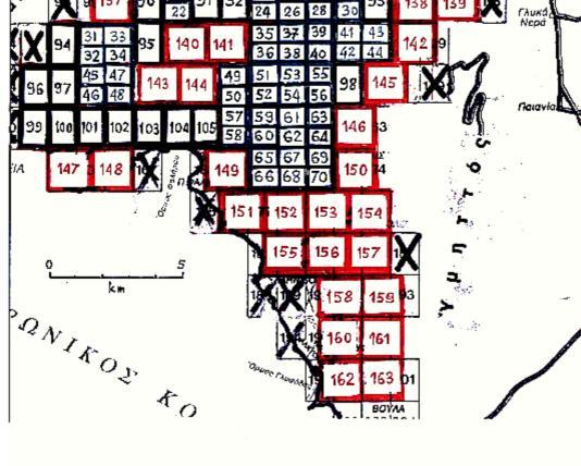
Grid construction for diffusive sampling measurements in an urban area (example of Athens)
