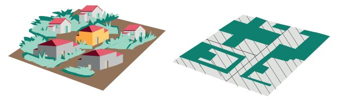
Figure 1.2. The relationship between land take (left) and soil sealing (right, hatched surfaces)
