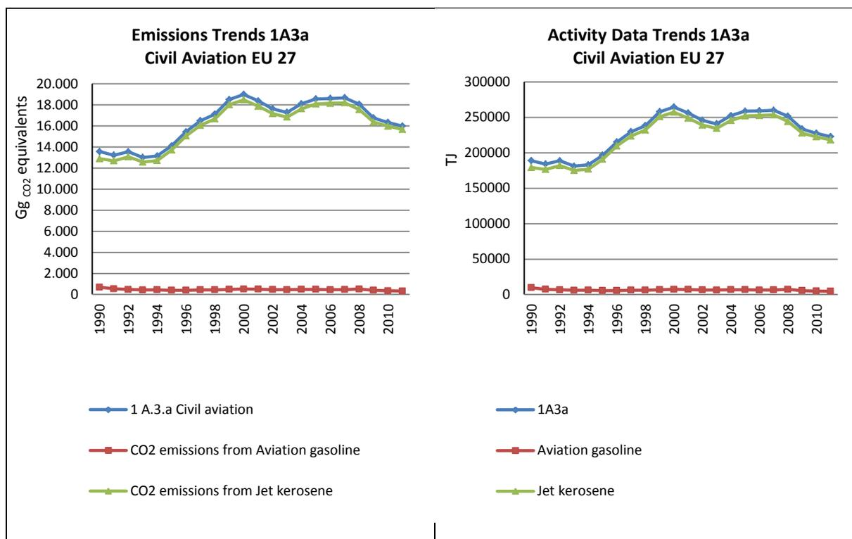
Table 18.29 1A3a Civil Aviation, jet kerosene: CO<sub>2</sub> emissions of EU-27
