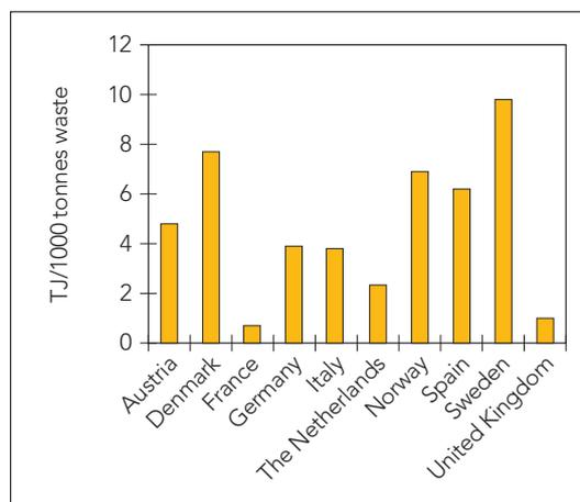
The figure shows a large variation among the EEA countries in total energy recovery (heat+electricity)/thousand tonne waste and is based on data obtained directly from the plants.
