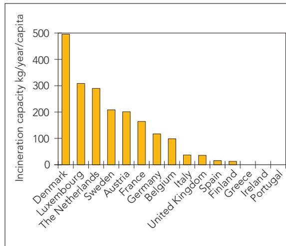
The figure illustrates a large variation in available incineration capacity per capita within the EU. The figure covers municipal solid waste incineration plants with and without energy recovery and is based on information on capacity where available or actual incinerated quantity in 1996 or the latest reported year before.
