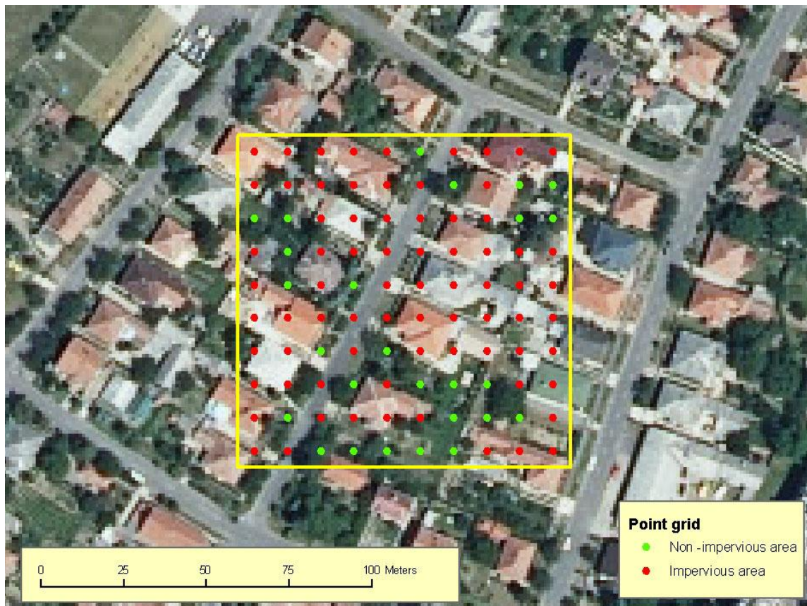
Figure 9 Validation methodology of European SSE data. By counting the number of impervious points inside the 100x100 m grid cell (total of 100 points), the interpreter estimates sealing degree of the sample cell.
