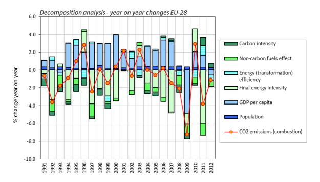
Note: The chart shows the estimated contributions of the various factors that have affected  $CO_2$  emissions from energy production and consumption in the EU-28. This approach is often used to portray the primary forces driving emissions. The explanatory factors should not be seen as fundamental factors in themselves nor should they be seen as independent of each other.
