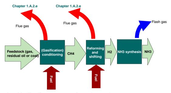
Figure 2.3 Simplified process scheme of ammonia production.
