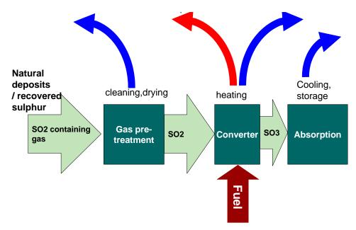
Figure 2.6 Process scheme sulphuric acid plant.
