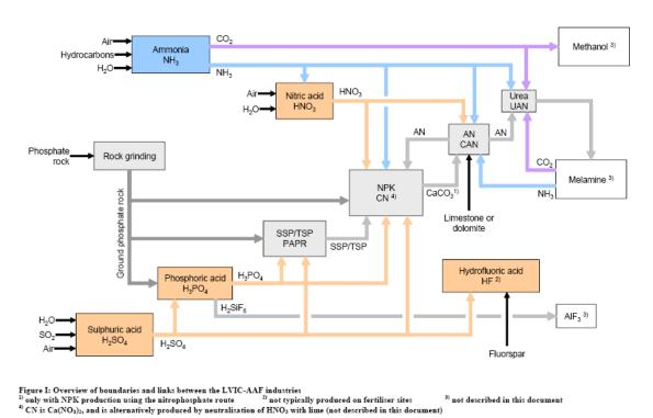
Figure 2.2 Example of integration of processes in the chemical industry (EC, 2006b).
