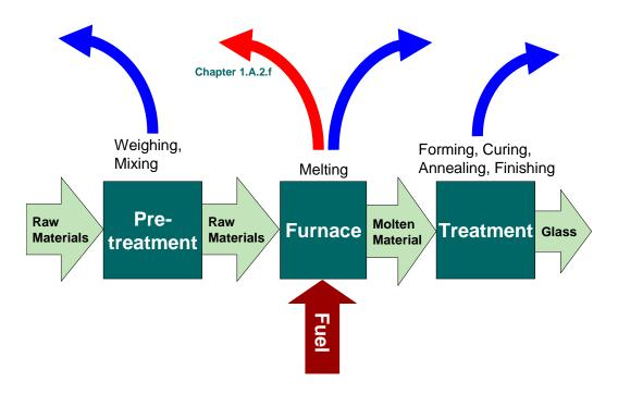
Figure 2.1 Process scheme for 2.A.3 Glass production, applicable for the production of glass.
