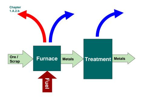
Figure 2.1 Generic process scheme for source category 2.C.5.e Other metal production
