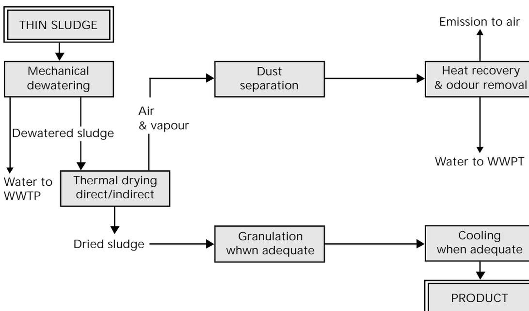
General flow sheet for a drying process
