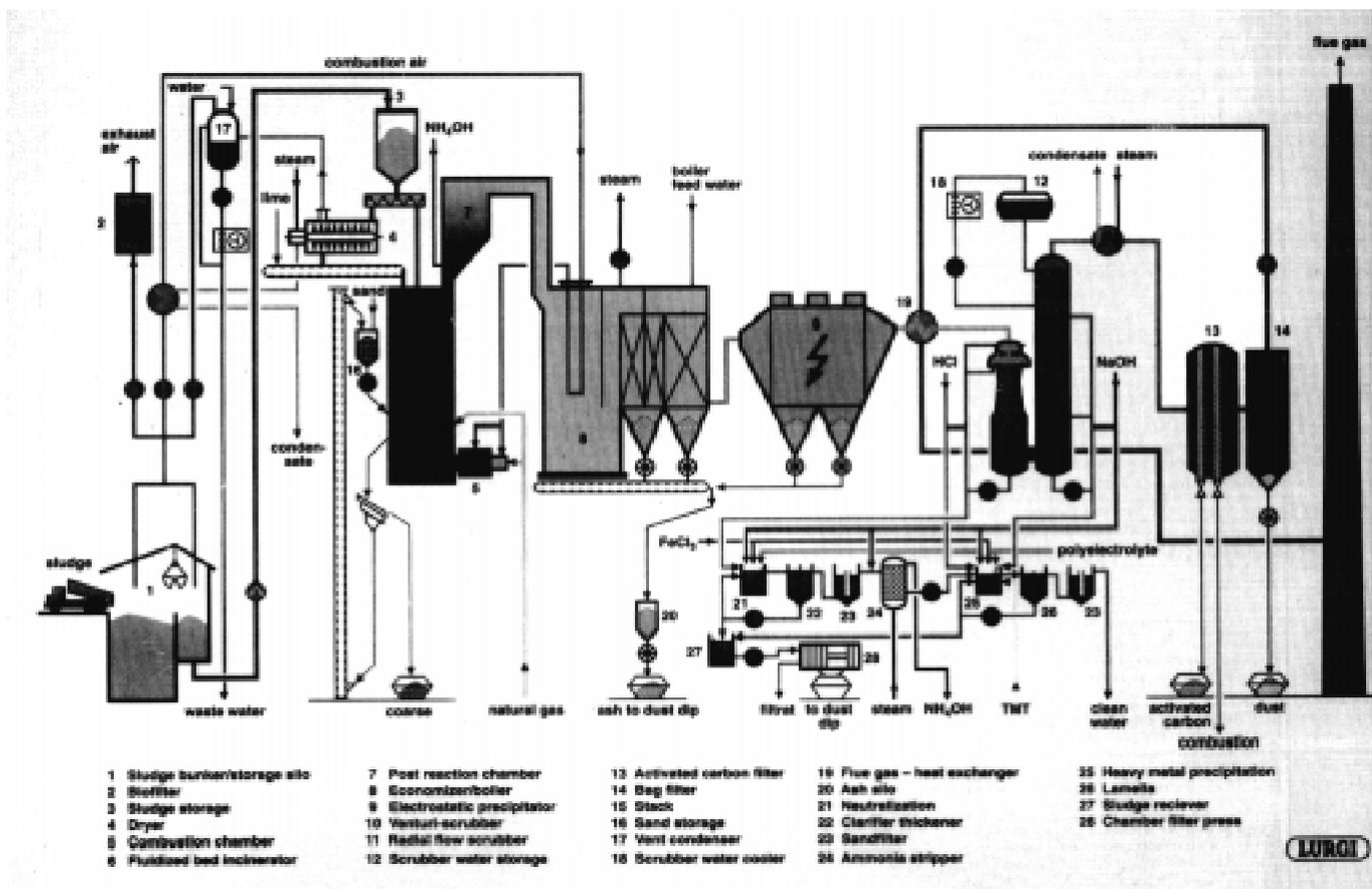
Process scheme of the sludge incineration plant of Dordrecht (the Netherlands)
